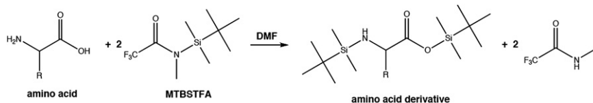
Fig. 1. Scheme of the derivatization reaction between a generic amino acid and MTBSTFA. A similar reaction will occur for carboxylic acids. DMF is used as the solvent.
